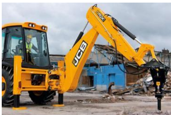
Figure 11: Example of Hydraulic hammer mounted on JCB-type excavator-loader.
